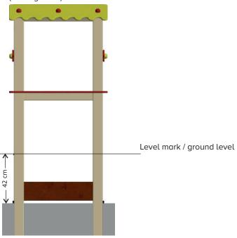
Installation on paving or rubber tilescaoutchouc (hard ground)
