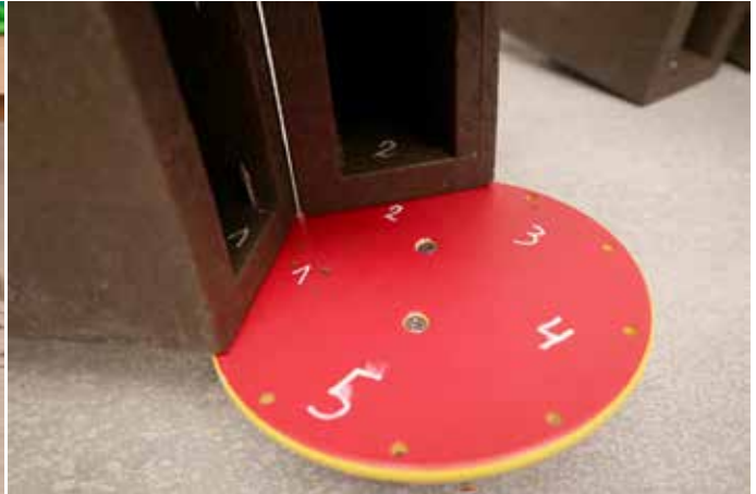
Screw the upper disc onto arm 1 (respect the numbering) and already place arm 2 between the discs
