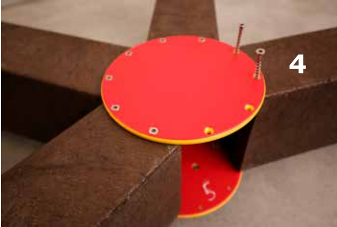
Screw the upper disc onto arm 4 and put this assembled part up, screw the lower disc to arm 4
