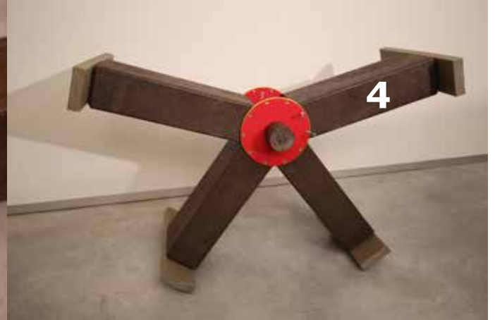
Screw the upper disc onto arm 4 and put this assembled part up, screw the lower disc to arm 4
