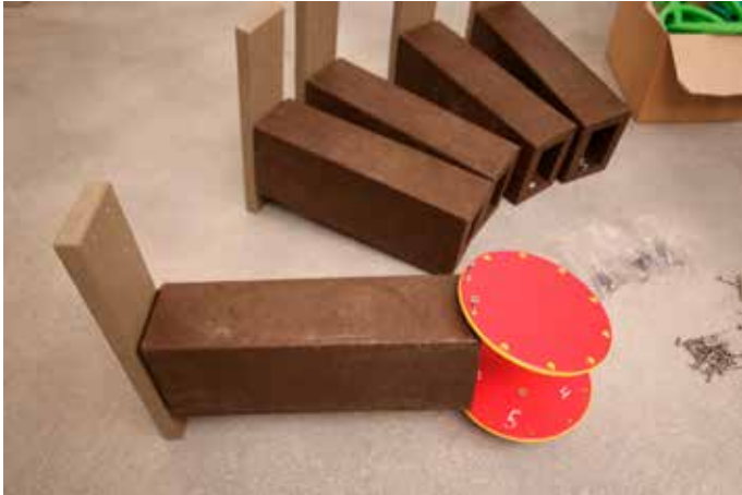
Screw the upper disc onto arm 1 (respect the numbering) and already place arm 2 between the discs
