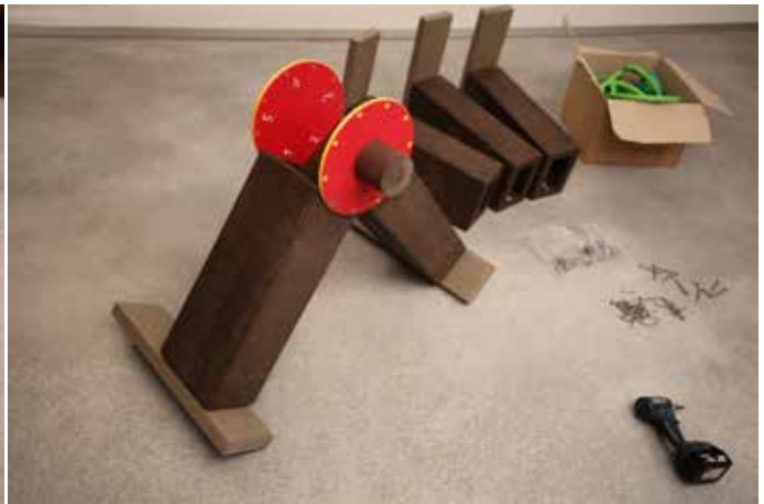
Screw the upper disc onto arm 1 (respect the numbering) and already place arm 2 between the discs
