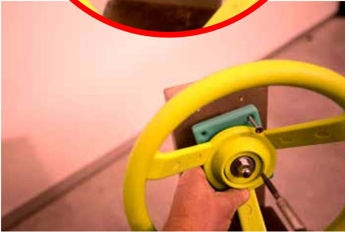
Screw the 10 steering wheels with the 40 countersunk stainless steel screws T25 with the plastic plate. The holes in the beige boards are marked with white markings.
