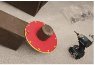
Turn arm n° 1 upside down and screw the lower disc with brown support onto the arm in the pre-drilled holes.
