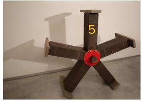
Screw the upper disc onto arm  $n^\circ\, 5$  and set upright, screw the lower disc onto arm  $n^\circ\, 5$
