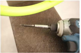
Secure the 10 steering wheels with the countersunk stainless steel screws T25 through the plastic plate. The holes in the beige boards are marked.
