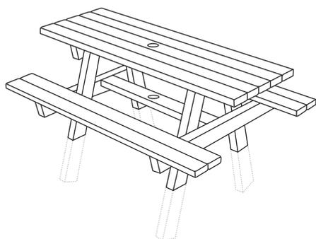
For safety reasons, it is recommended to respect at least 10 cm between the top of the anchorage (concrete) and the ground level. Required volume of concrete per table leg: +/- 0,15m<sup>3</sup>
