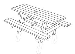
For safety reasons, it is recommended to respect at least 10 cm between the top of the anchorage (concrete) and the ground level. Required volume of concrete per table leg: +/- 0,15m<sup>3</sup>
