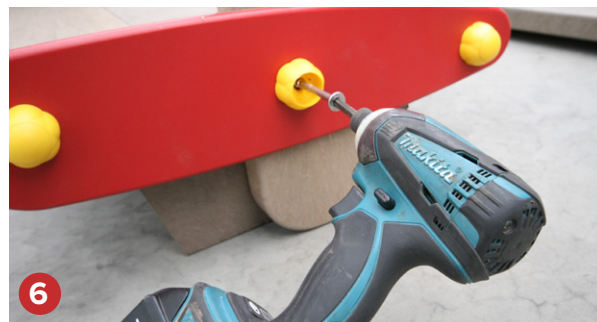
Mount the wing supports with the 2 supplied screws 8 x 120 (Torx 40) and the 2 yellow cover caps
