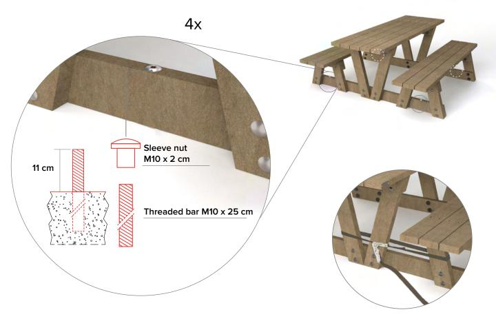
tip: use a tie down strap to align the fixation holes
